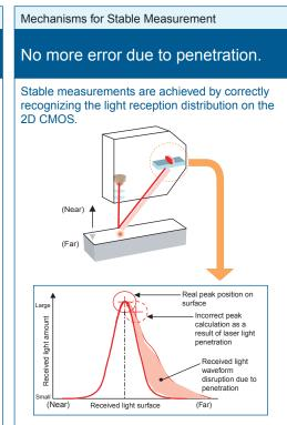
Real surface displacement detected by eliminating penetration effects for PCBs, plastic, and other workpieces penetrated by laser light.
